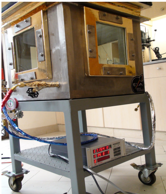
The Space Environment Simulation Chamber- SESCA
