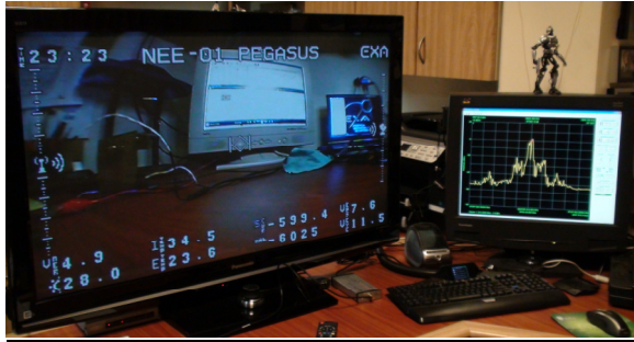
Image of the NEE-01 PEGASUS video transmissions with the OSD telemetry
