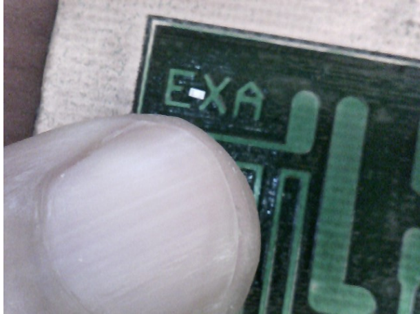
Detail of a 1pF condenser integrated into the TX amplifier, soldered manually
