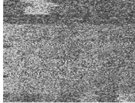
A P0-quality video signal level, Signal/Noise ratio of <3 db, <5 microvolt signal strength.
