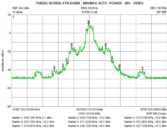
The NEE-01 PEGASUS signal graph for video/audio transmission, signal as an input attenuation of 20dB in order to avoid damage to the oscilloscope.
