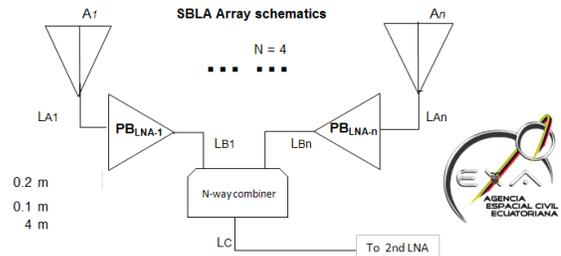
The main concept in the SBLA array is that of an antenna farm or a big virtual antenna, but with short baseline, coupled with the PBLNA technique, gives out a powerful amplification gain with minimal signal blurring.
