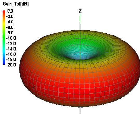
The NEE-01 PEGASUS dipole radiation pattern, which actually is tilted 90 degrees
