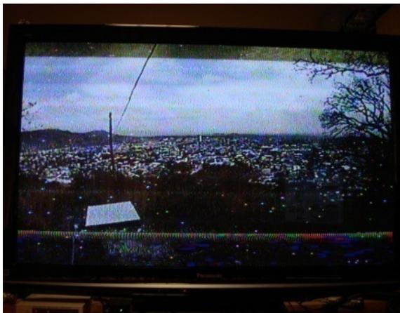
*The resulting signal from 20.5kms away, using phase F0 of the ARGOS manifold, the transmitting source was at 0.002W TX power, some interference can be observed due other sources in the vicinity.*
