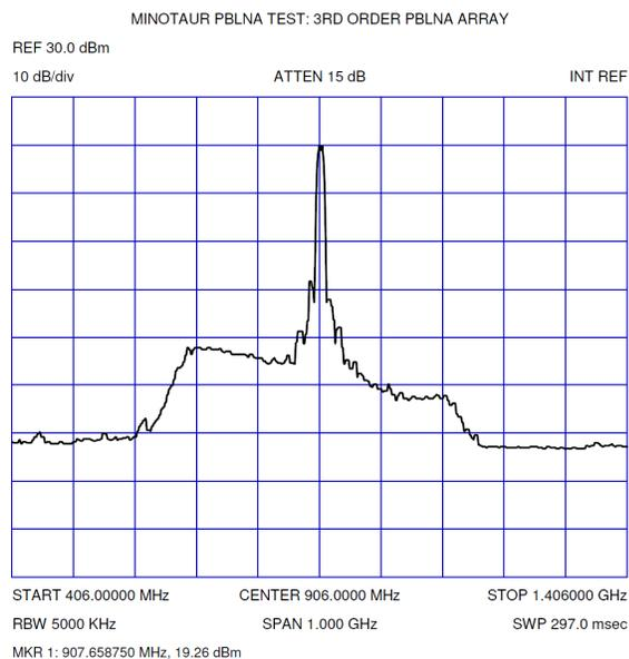
*The resulting amplified signal with 240dB physical attenuation, the internal oscilloscope attenuation was set to 15dB to avoid damaging the device. Signal level was 19.26dB*
