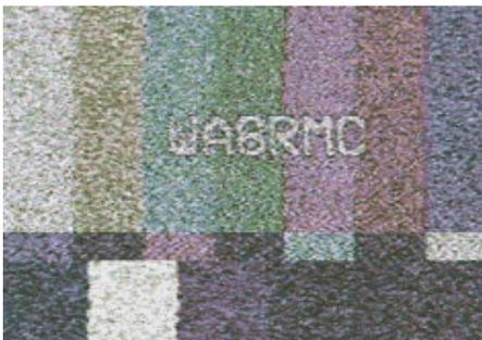
A P2-quality video signal level, Signal/Noise ratio of 8-20 db, 15-50 microvolt signal strength.
