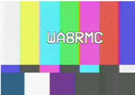
A P5-quality video signal level, Signal/Noise ratio of >45 db, >1000 microvolt signal strength.
