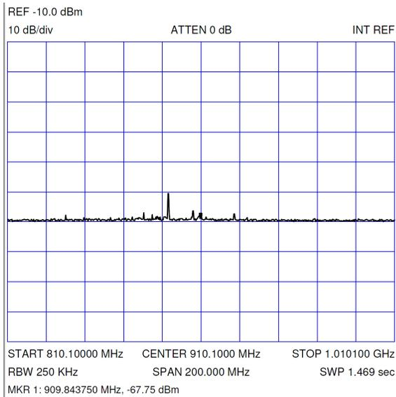
*The originating signal at 1W with 240dB physical attenuation, the internal oscilloscope attenuation was set to 0dB, the signal level was -67.75dB*
