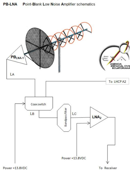
The idea behind the PBLNA is to have a series of LNAs as near as possible of the reception point in the antenna to minimize losses, this approach is very
