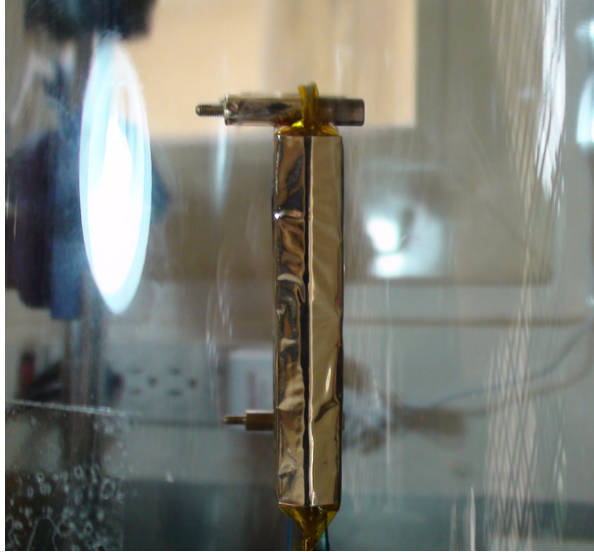
Fig-12 Final battery array in a 3.6 \times 10^{-6} mbar vacuum environment showing negligible or no swelling at all.
