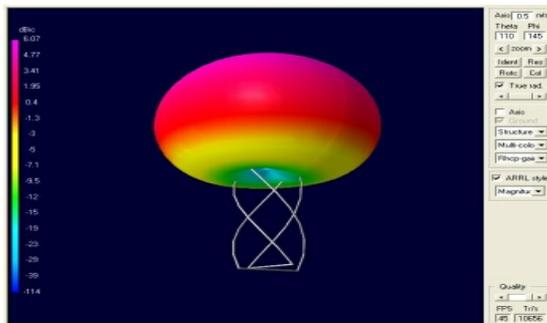
Fig. 6: QHA RHCP radiation pattern. Adapted from <http://homepages.ipact.nl/~pa1are/QHA.html><sup>16</sup>
