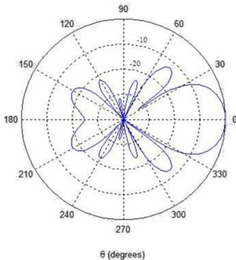
Fig. 3: MINOTAUR antenna radiation patterns
