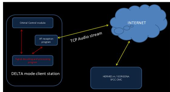
Fig. 5: HERMES Delta mode client station. The APT from NOAA is received and relayed to remote users in real-time through Internet
