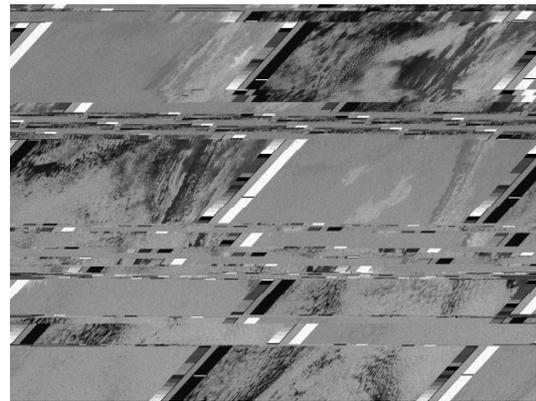
Fig. 15: Image is 'slanted' due to under-sampling frequency and has 'Synchronization losses' due to high priority program running on the machine.
