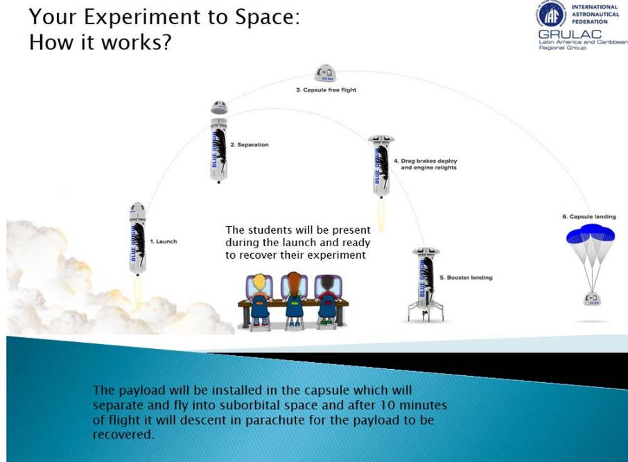
Figure 1 – New Shepard Trajectory (courtesy of blue origin)
