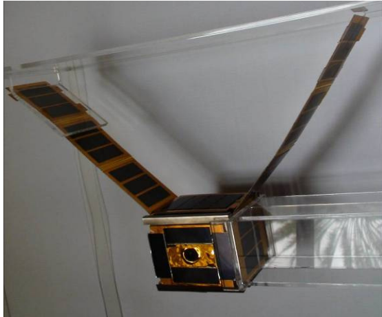
Fig-4 The NEE-02 KRYSAOR in orbital flight configuration with its 2 DSA Multipanel solar wings deployed
