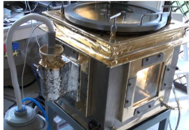
Fig-16 the latest working design of the SESCO chamber shown in operation with both the cryogenic (KRYOQVANT) and thermal (HELIOS) modules at the same time.
