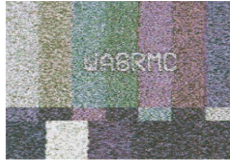
Fig-14 A P2-quality video signal level, Signal/Noise ratio of 8-20 db, 15-50 microvolt signal strength.
