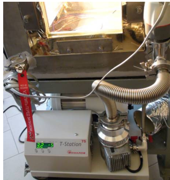
Fig-17 Detail of the vacuum pump operating in mid-thermal vacuum, with the temperature inside the chamber over 200C.
