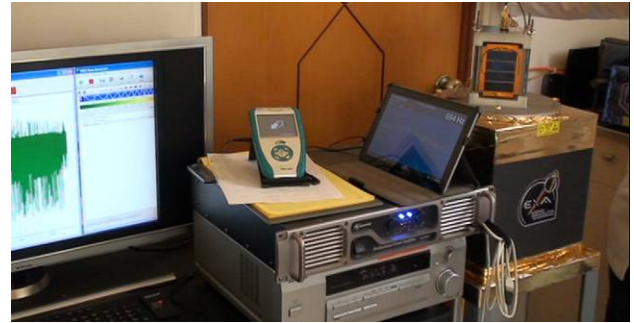
Fig-22 The NEE-01 flight model being subject to LSP vibration tests on the GOLEM magneto dynamical shaker facility.
