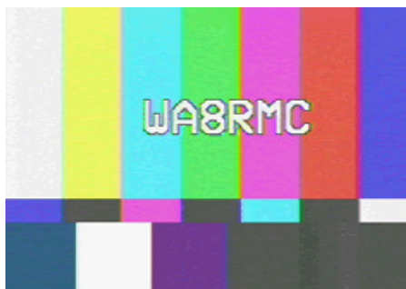
Fig-13 A P5-quality video signal level, Signal/Noise ratio of >45 db, >1000 microvolt signal strength.
