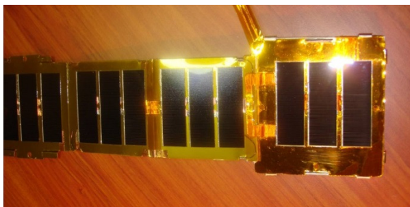
Fig-5 One of the DSA solar arrays with its 99.98% pure titanium scaffolds of 0.25mm and the SEAM/NEMEA shield
