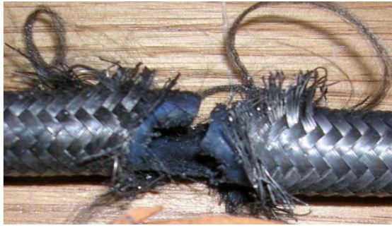
Fig-14.1 Example of damage caused by a 1 mm size particle on a satellite electrical cable. See reference #47
