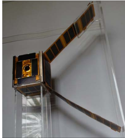
Fig-2 The NEE-02 KRYSOR in orbital flight configuration with its 2 DSA Multipanel solar wings deployed
